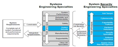
Figure 9: System engineering and system security engineering trade-offs
